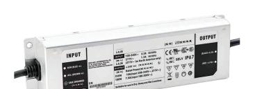
PSDE-180W-24V-010 is a 240W AC/DC LED driver that features a high-efficiency output of 93% allows it to operate under free air convection. The metal housing design and IP67/65 ingress protection rating makes it suitable for both indoor and outdoor use. It has dimming functions, adjustable output, and built-in active PFC.
